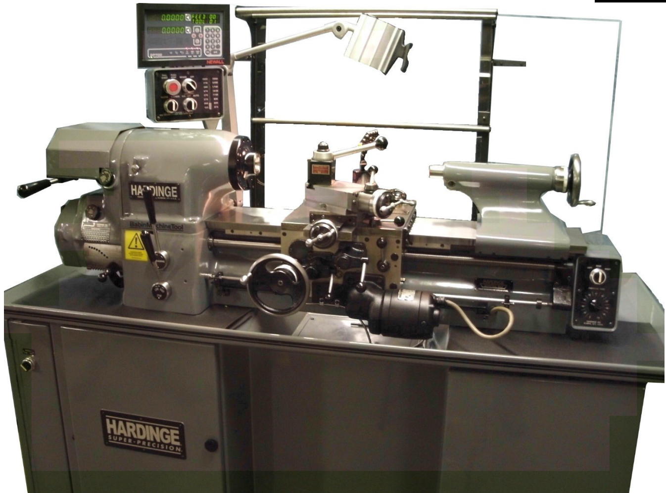
1979 HLV-H-toolroom lathe rebuilt with .0001"res Newall DP700 DRO
